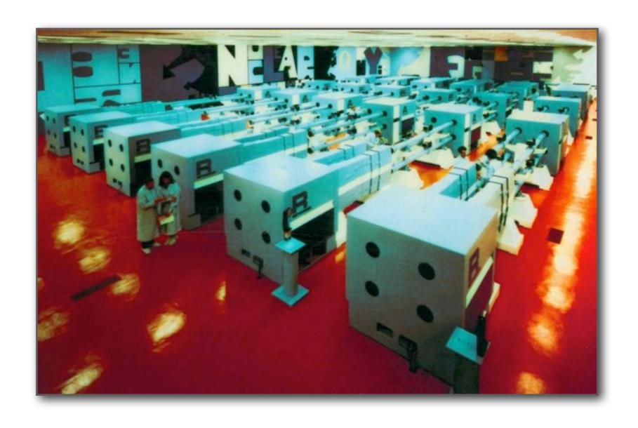
LLE Facility's Omega Laser System laser bay. The Omega Laser produced peak power 12 terawatts and maximum energy per pulse of 10 kilojoules which could be focused on a 100 µm diameter fuel pellet to initiate laser driven fusion reactions.
