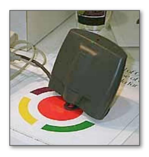
The Colortron, developed by the Optel Team while at Lucid, Inc., was the lowest cost (\$325) OEM price) 32 spectral band color measurement instrument ever produced. It rivaled the performance of devices costing thousands of dollars more. The Colortron was custom designed and manufactured for Light Source Computer Images by Lucid and the device won numerous design awards in the graphics arts industry. Lucid manufactured approximately 15,000 of these devices over the product's life.
