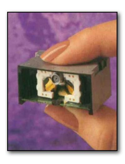
The DI-1000 barcode scanning module was designed specifically for manufacturers of portable data collection terminals. It was small enough to fit inside the enclosure of a handheld data collection terminal and was intended to eliminate the need for a separate handheld barcode scanner attached to the portable data collection terminal via a cable. The DI-1000 was designed to avoid all of the patents of in the crowded IP space of the very litigious bar code industry.
